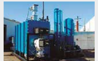
Thermolysis Plant: 1,7 g/h with SUW, 3,9 g/h with plastic.
